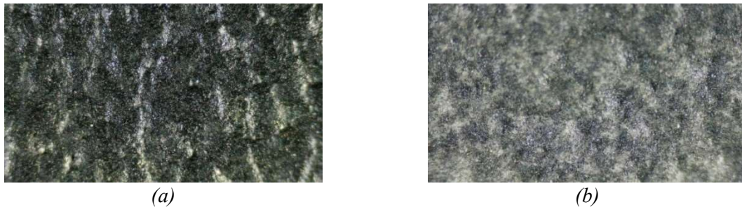
Figure 5 - Surface of G7Nan (a) and G2Nan (b) nanocomposite base coats
